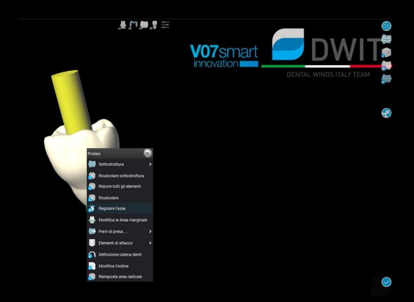
ADJUSTMENT OF THE AXIS OF THE INCLINED HOLE WITH THE ROTATION OF INTERFACE
